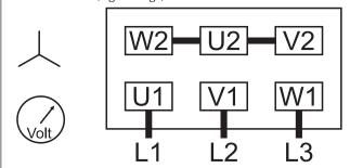
Double star connection, multi-voltage motor (low voltage):
